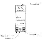
indication of input, output and power of the IsoBlock I-FG
